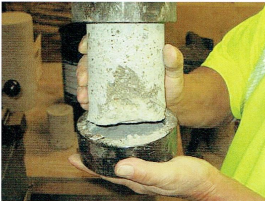
Fig. 3: Type of break indicative of a point load as a result of a core that has not been cut to 90 degrees
