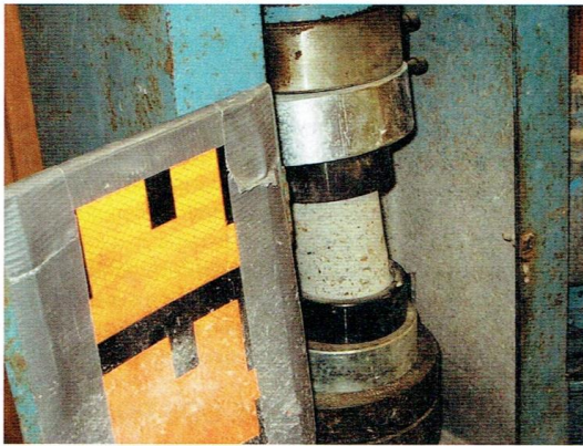
Fig. 2: Specimen that has not been cut to 90 degrees in a break machine
