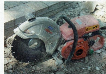
A wet saw, available at most rental outlets, is the most productive means of cutting pavers.
