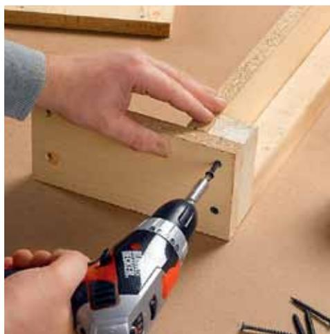
2. Fasten the end panels to the end blocking with 2" screws. Install the bottom panel with screws driven through the panel and into the bottom blocking. Make sure all panels and blocking are flush along the top and bottom edges. Note: You may need to leave one end open in order to work, as we have done here.
