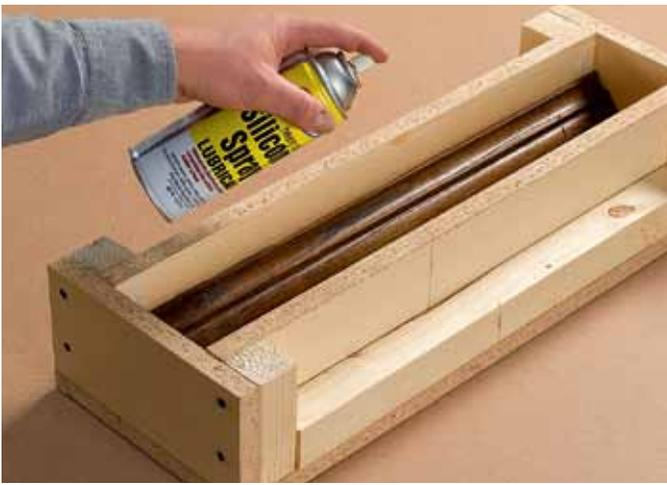
4. Coat the inside of the mold (all nonmelamine parts) with clean vegetable oil or another release agent. Mix a batch of concrete following the product directions. An 80 lb. bag of crack-resistant concrete will fill two of the molds.
