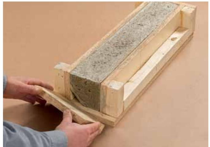
7. Carefully disassemble the mold by unscrewing the ends and bottom from the sides, as needed. Scrape, file, or grind any ragged edges for clean detailing in the finished piece. For maximum strength, set the casting in a shaded area and moisture-cure it for three to five days, keeping it damp under plastic sheeting.
