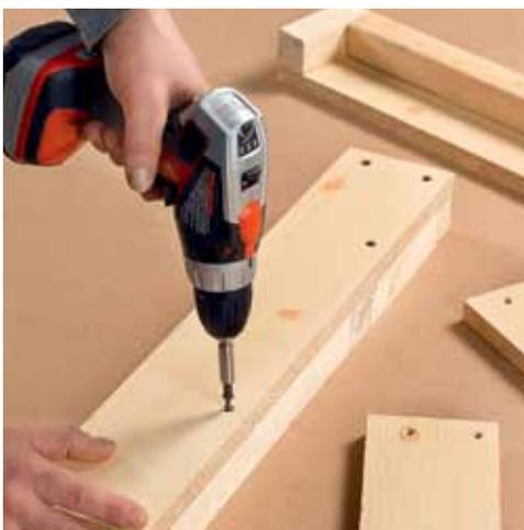
1. Cut the pieces for the mold. Fasten the end blocking pieces flush with the ends of the side panels using pairs of 2" drywall screws driven through pilot holes. Fasten the bottom blocking to the side panels, flush along the bottom edges.
