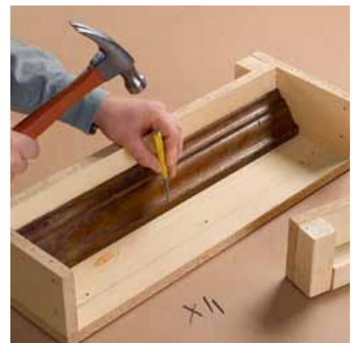
3. Add trim or other elements as desired for custom shaping effects. Here, we used crown molding, which we fastened to the blocking with finish nails using a nail set. Cover the screw heads on the inside of the mold with silicone caulk; then flatten to create a smooth, flat surface.
