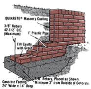
As with the concrete retaining walls discussed on page 16, brick, block, and stone retaining walls protect your property from soil erosion while, at the same time, adding distinction to your home's exterior. The building procedures are the same as those used in basic wall construction; refer to the Footers, Basic Brick Construction, Concrete Block Construction, and Stone Masonry sections for details. The tools and
