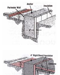
**1.** Dig a 2' (0.6m) wide footer trench to a depth several inches below the frost line. In firm soil, one side of the trench can act as a form. Construct and install the outer and inner form walls as shown.
