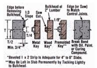
They can be hand tooled in fresh concrete or sawn into hardened concrete. Control joints should penetrate roughly ¼ of the slab thickness and be spaced every 6' to 8' in 4"-thick slab work. Wide driveways and patios may require longitudinal control joints down their centers. Expansion joints help dissipate the expansion and contraction forces that pass between adjoining structures.
