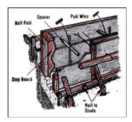
**5.** Strike off the concrete flush with the top of the form. Float and trowel it to the desired finish. Insert anchor bolts for mud sills and wooden caps once the concrete has set sufficiently to hold them.
