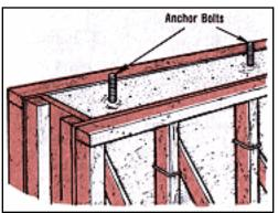
**8.** As each section is poured, allow it to set (12 to 24 hours) before removing the stop board. Before pouring the new section, coat the exposed end with QUIKRETE® Concrete Bonding Adhesive to avoid leaks caused by the cold joint. For Best Results: Make curved forms by nailing multiple strips of saw-kerfed plywood or semiflexible hardboard to the form studding.
