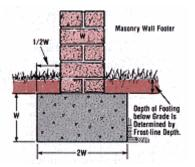
**2.** Firmly compact the soil using a tamper, and add 6" of QUIKRETE® All-Purpose Gravel or crushed stone to the base to ensure good drainage.
