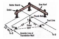
2. Transfer the building lines to the batterboards by dangling a plumb bob over the outer edge of each corner stake while stretching a length of line between batter boards. This is best done as a two-person operation.
