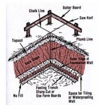
**4.** After digging the trench, a plumb bob can be used to transfer dimensions for footer forms and final wall positions.
