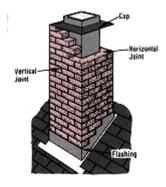
Although repairing a leaning chimney or one that is leaking smoke through the brick joints are jobs best left to a professional, there are some important repairs that anyone can perform. These include repairs to preserve the integrity of the brickwork and to avoid more serious and expensive work in the future. If your chimney has crumbling pointing or holes and cracks in the cap, doing the repairs yourself immediately
