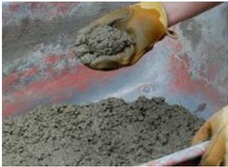
**Properly mixed concrete should look like thick oatmeal and should hold its shape when it is squeezed in a gloved hand.**
