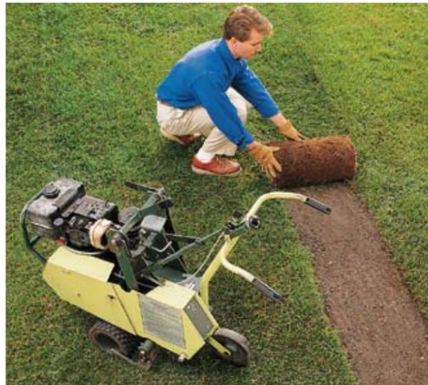
■ **Use a sod cutter** to strip grass from your pathway site. Available at most rental centers, sod cutters excavate to a very even depth. The cut sod can be replanted in other parts of your lawn.
