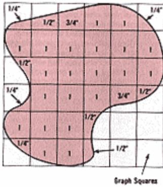
designs is that the amount of usable patio space is reduced. For example, a square patio measuring 20' (6m) on a side provides 400 square feet ( $37m^2$ ) of surface area, while a circular patio with a diameter of 20' (6m) provides only about 315 square feet ( $37m^2$ ) of surface area.
