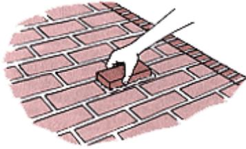
4. Strike the tops of the joints flat to prevent water entry. After the mortar is dry enough to be brushed without smearing, brush away any loose particles of mortar.
