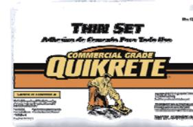
approximately 6-6.5 quarts (5.6-6.2 L) of water per 50 pound (22.7 Kg) bag. Do not use high-speed, high-shear type equipment for mixing. Mix thoroughly and let stand for 10 minutes. Remix before use.
