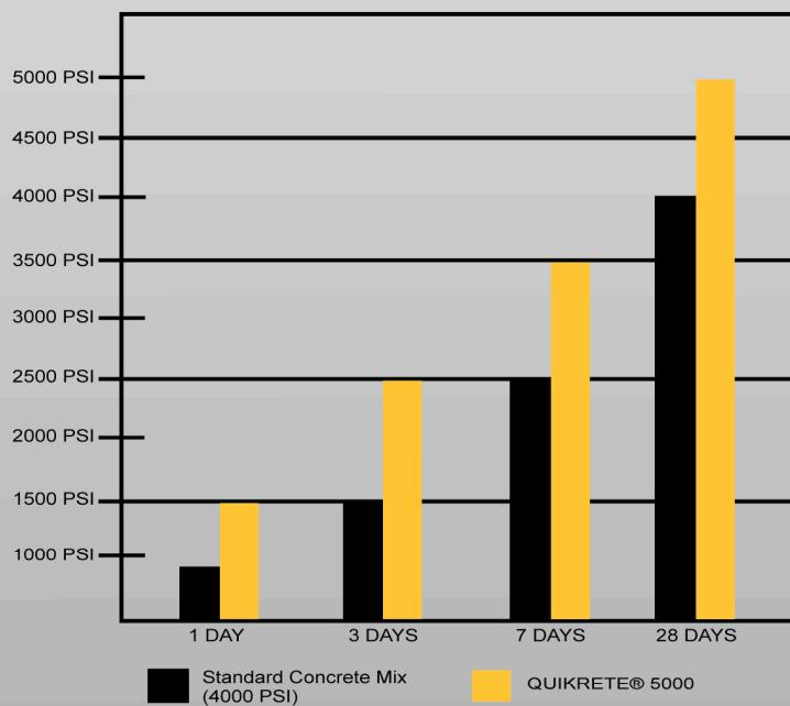
Note: Regular QUIKRETE® Concrete Mix (Product #1101-yellow bag) is designed to meet the compressive strength requirements for standard concrete per ASTM C387.
