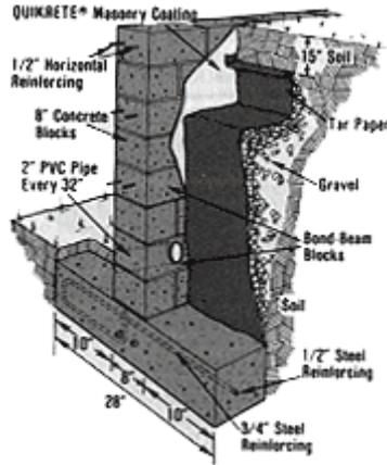
Notch the brick/block to accommodate the pipes and use a mortar to secure them as shown in the illustration. On the stone walls, slope the pipe downward toward the front of the wall, about 8" above the front grade; this will prevent pressure buildup against the back of the wall. Place a screen over the back opening and pile broken stone over the screen to prevent the pipe from becoming clogged.
