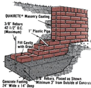
As with the concrete retaining walls discussed on page 16, brick, block, and stone retaining walls protect your property from soil erosion while, at the same time, adding distinction to your home's exterior. The building procedures are the same as those used in basic wall construction; refer to the *Footers, Basic Brick Construction, Concrete Block Construction, and Stone Masonry* sections for details. The tools and
