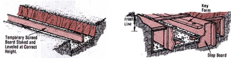
**7.** On slopes, construct a stepped footing to minimize the amount of concrete used. Stepped forms should rise no more than 2' per step and overlap at least 2' at each step. The same step principle can be used for earth forms.
