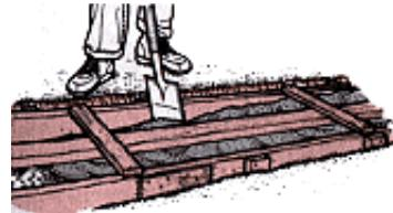
**2.** Screeed the concrete level. If steel reinforcement is needed for the poured wall, insert it at this time. Predrilled holes in the keyway form make this an easy task. Remove the keyway form as soon as the concrete has set up sufficiently to hold its shape.
