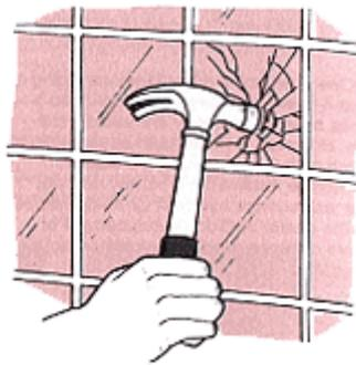
2. If you are replacing an entire section of tile, use a hammer and a straight bar or chisel to loosen the top tile. It should work free by tapping lightly with the hammer. Work down and remove the rest of the tile in the same manner.
