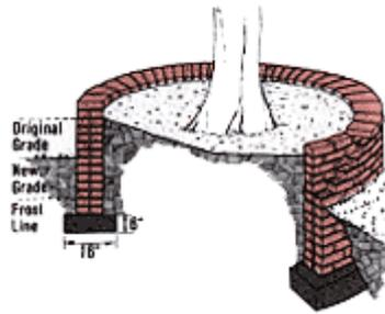
3. Excavate a 16"-wide trench, beginning about 4" inside the hose. Dig the trench to several inches below the frost line, keeping the bottom 6" of the trench as smooth as possible so that a footer can be poured without constructing forms.
